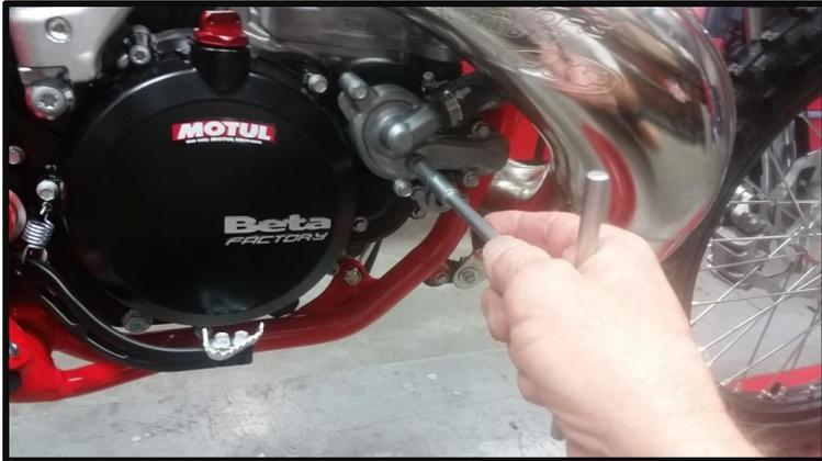
When the engine is cold, remove the radiator cap and drain the coolant into a clean container.
