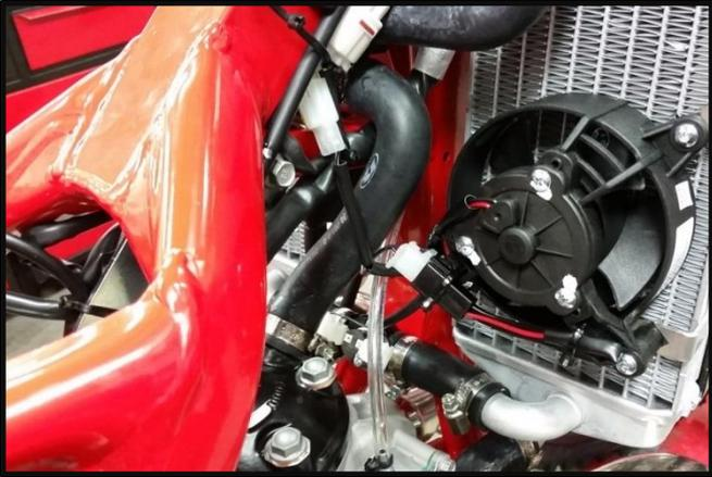
Reinstall the radiator along with the lower cooling hose. Plug the fan wires into the thermoswitch loom and then plug the remaining plug from the thermoswitch loom into the main harness of the motorcycle. Ziptie the wires to the fan as shown.
