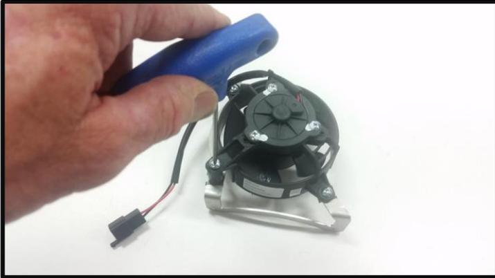
Install the fan motor using the three nutclips and screws provided as shown in the photo
