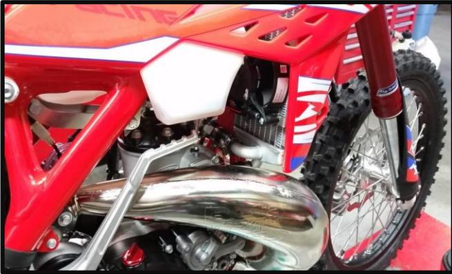
Reinstall the fuel tank, fill the radiator with coolant making sure the coolant system has been bled. Reconnect the battery.
