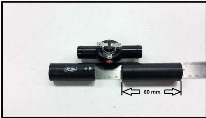
Cut out 35mm from the lower cooling hose to allow room for the thermoswitch assembly making sure that one of the hoses is roughly 60mm in length as shown.
