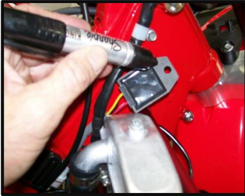
Having already removed the 6mm bolt from the frame. Take a marker and put ink on the positioning nub. Using the bolt hole as a guide, reposition it where it clears the radiator guards and press it against the frame making an ink mark .
