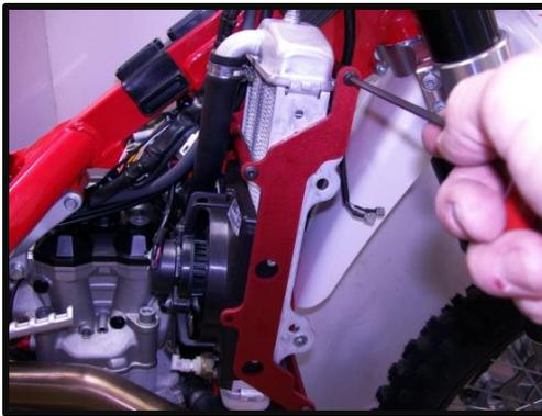
8) Install the outer right side plate using 6mm button head allen bolts.
