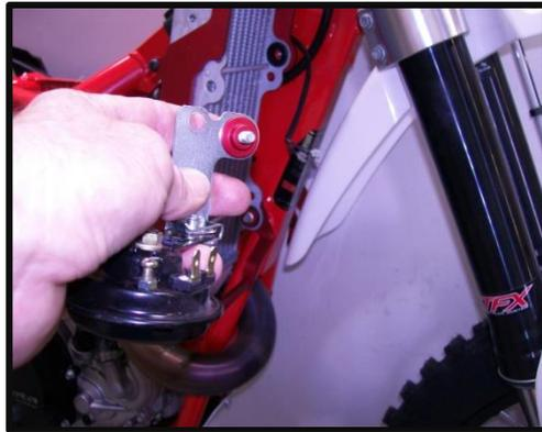
7) Place one of the supplied 6mm bolts through the horn bracket then a hat washer. Install through the top radiator and brace mounting holes and secure to the frame and torque to 10 newton meters. Repeat using a 6mm bolt and hat washer on the bottom mount.
