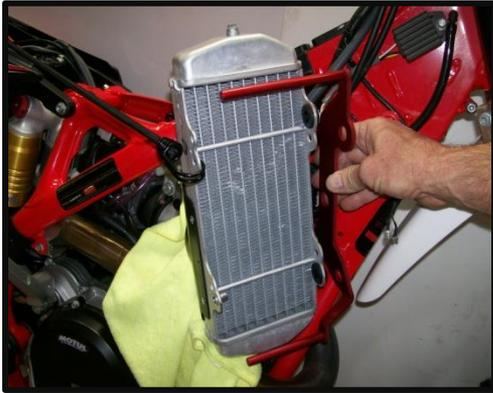
6) Disconnect the horn wires and remove the 2 - 6mm bolts, horn and washers holding the right side radiator to the frame.
